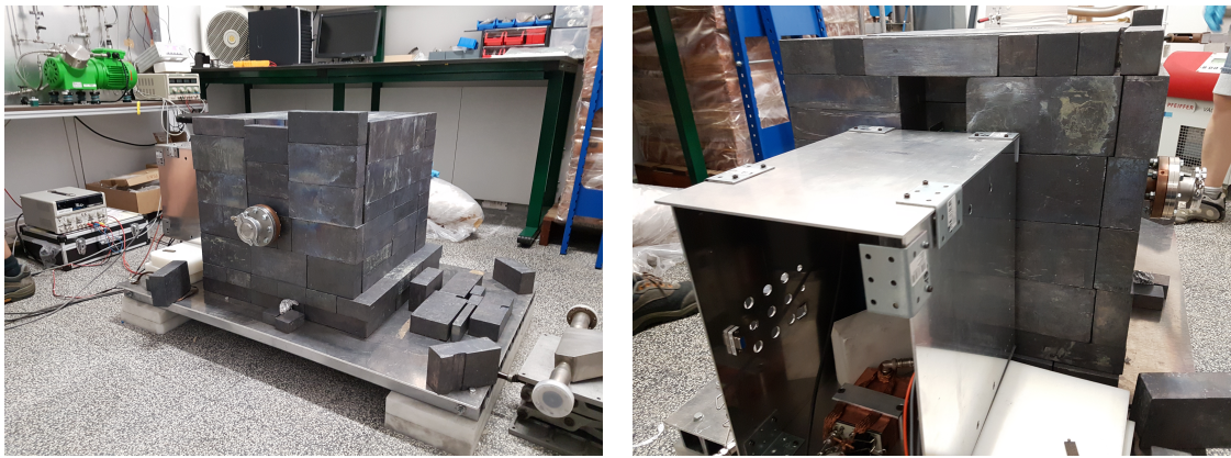
Figure 8.14: (Left) Picture of the lead passive shielding of IAXO-D0. (Right) Picture of the side of the shielding where the electronic connections are placed. This is one of the weak spots of the shielding.
