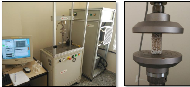
Figure 15: On the left, servo-hydraulic material testing machine; on the right, uniaxial compression test
