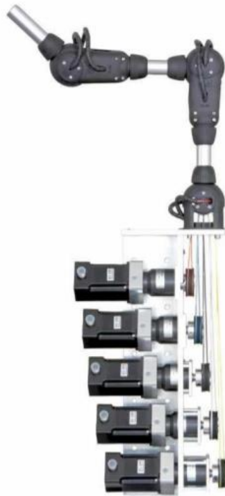
Figure 3.1. System cable driven joints. [Igu19]
