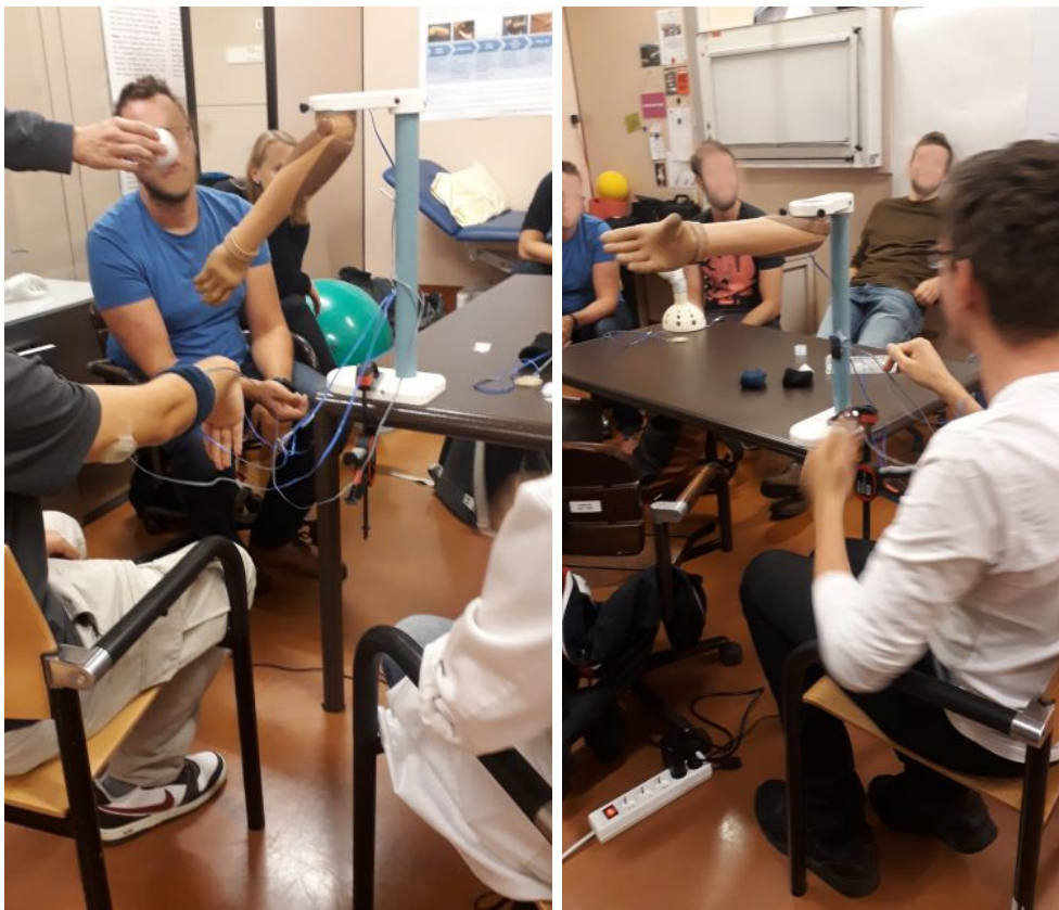
Figure 2.5: Students trying the bionic hand. In the image on the left each of the students is controlling one movement of the bionic hand, one of them the arm lifting and the other one the hand opening. In the image on the right one student is trying to throw the ball.
