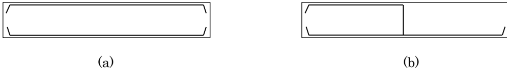
Figure 7. Different capillaries designed for the project. (a) Straight capillary. (b) “Chair size” capillary.
