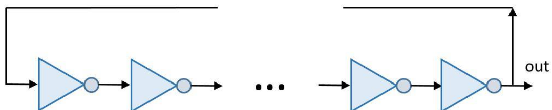
Fig. 4.6. Scheme of a ring oscillator. The number of inverters must be odd.
