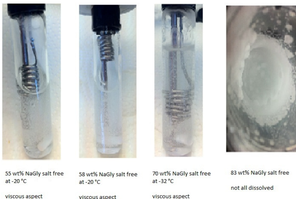
Figure 29. Some solutions of sodium hydroxide and glycine with a nNaOH/nGly relation (1:1) in water.
