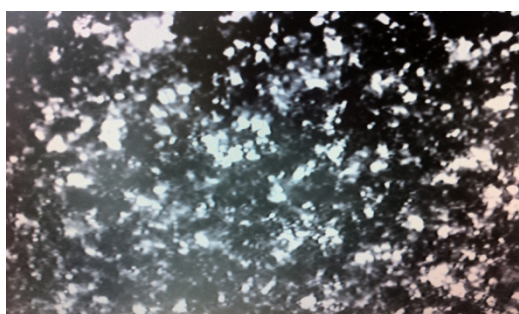
Figure 86. Crystals seen in the microscope for the solution 27.5 wt% \text{KHCO}_3 .
