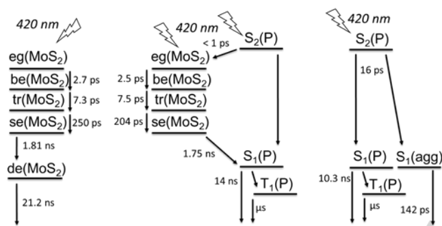
Figure 6. Deactivation models for MoS 2 (left), 2 (middle) and 1 (right) upon 420 nm excitation.
