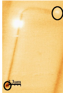
Figure 38: The circles show the magnetic flux coming in and out due to the single-domain state existing in this wire. The other contrast changes are produced by the topography.
