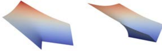
Figure 1: Geometrical singularities: solution of the Poisson equation for a domain with reentrant corner (left) and slit domain (right).
