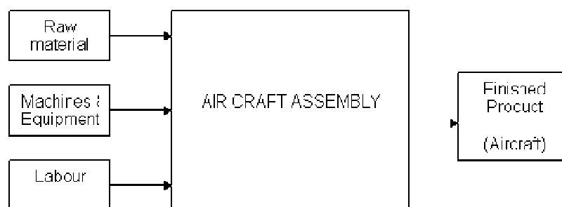
Figure 39 Fixed position or location layout
