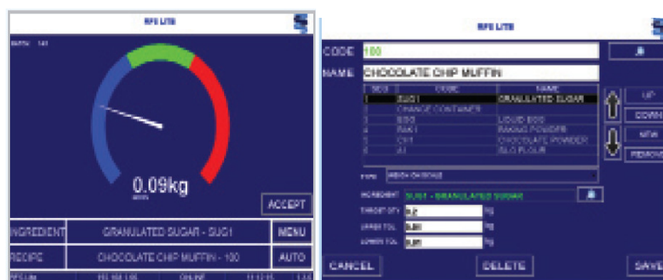
Figure 33 Stevens Vantage interface formulation system (weighing ingredients)
