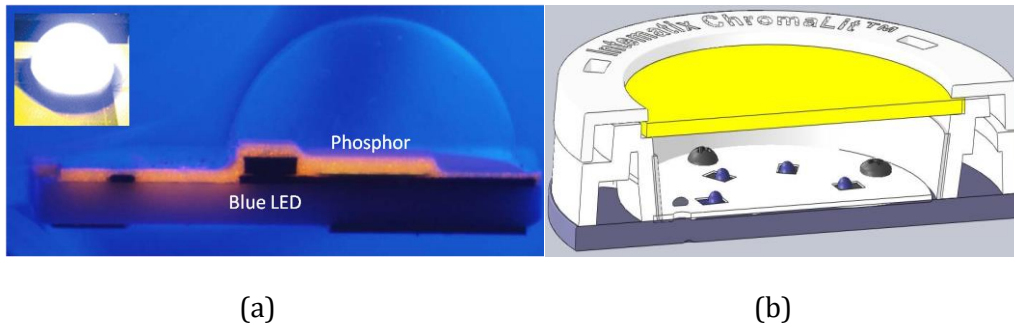
Figure I.3. Philips Lumileds HB-LEDs with package level conformal coating (a) and Intematix ChromaLit light source with remote phosphor configuration (b).
