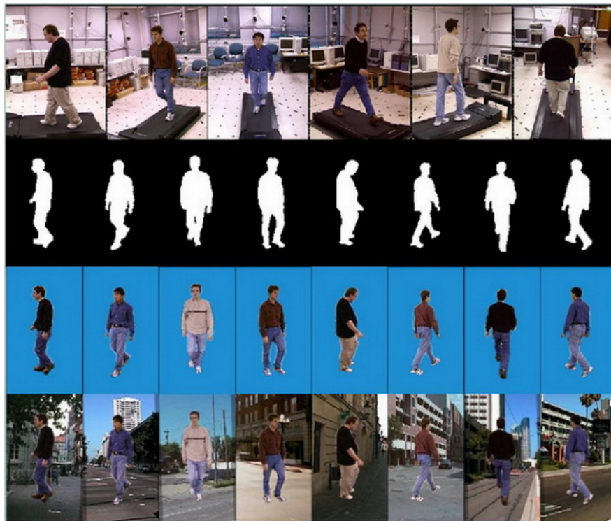
Figure 6.12: Modified MoBo dataset ( from top to bottom ): we show an original image for each one of the 6 available camera views ( 1st row ). We then present a normalized 96 \times 160 binary segmentation per training view ( 2nd row ), the corresponding segmented images ( 3rd row ) and images with a random background ( 4th row ).
