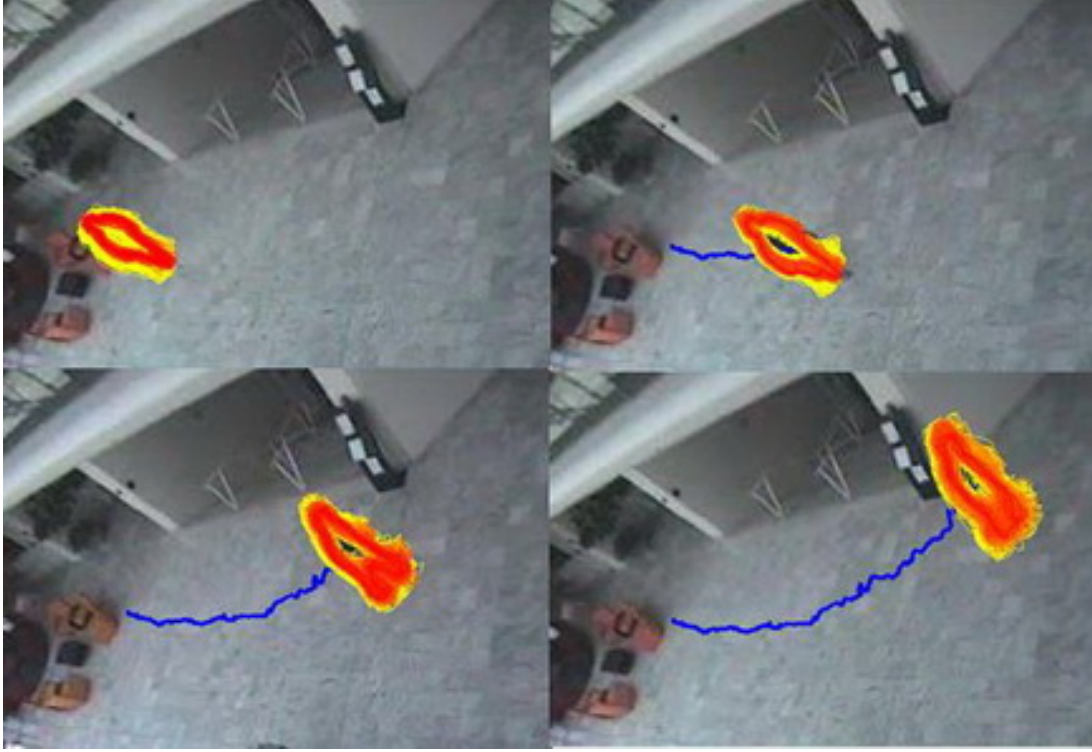
Figure 5.6: Visualization of the likelihood for the entire sample set in several frames of the Walk2 sequence. For each frame, we plot the set of sampled and aligned shapes: darker colors indicate a higher likelihood.
