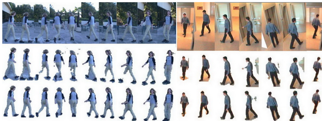
Figure 3.10: Segmentation results for (left) “Walkcircle” outdoor sequence and (right) for “elevator” indoor sequence. (up) the original image, (centre) the result obtained by simple background subtraction and (down) the result obtained by applying the proposed model-based algorithm are represented for each example.
