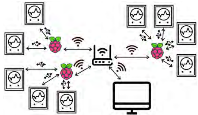
Fig. 1. Hardware connection scheme for the wireless control: Both the host computer and the Raspberry-based gateways are connected to a Wi-Fi network (previously available in the measurement area, or ad hoc). Gateways send commands and queries received from the host to the instruments through their USB buses, returning the corresponding instrument messages to the computer.
