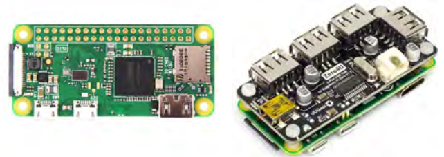
Fig. 2. (left) Raspberry Pi Zero W top view. (right) Zero4U coupled to the Raspberry Pi Zero W.
