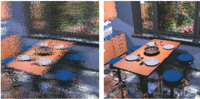
Figure 4.12: Images generated using frameless rendering. Left, naive frameless rendering where each sample is displayed as soon as is calculated. Right, the same image using adaptive frameless rendering [55]
