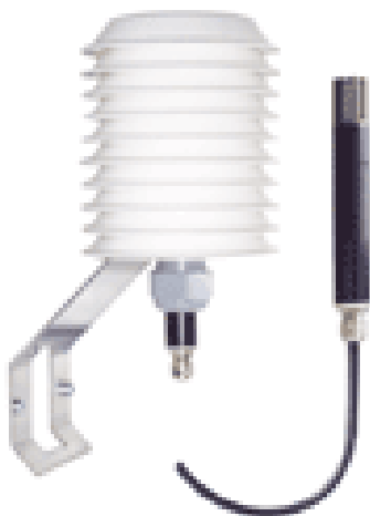
Figure 29: Relative humidity sensor (left) and temperature sensor (right) /1/
