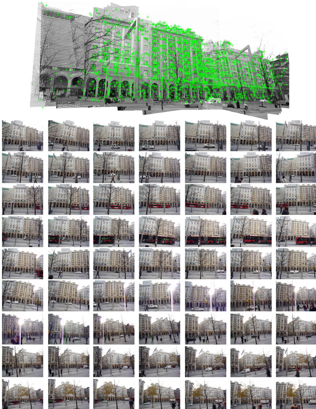
Figure 6.4: Planar region extracted from one sequence of the Downtown data set. The algorithm is able to track and grow the plane over 63 different frames with dynamic elements and some illumination changes. The top figure represents the plane with the 482 detected features. The plane has been observed in all the images depicted below.
