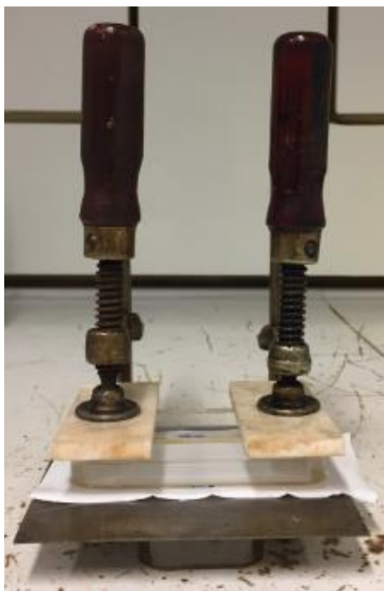
Figure A-4. In house developed interfacial polymerization set-up
