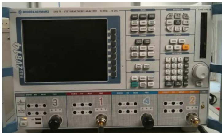
Figure 10: Network analyzer employed to measure the transmission.
