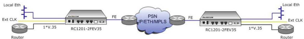
Figure.1 PTP Application for V.35 Data Transmission
